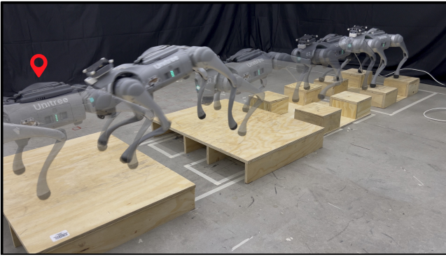
Figure 15. Hardware experiment demonstration for the second unstructured terrain scenario with sparse stepping stones, flat, and gap terrains.
