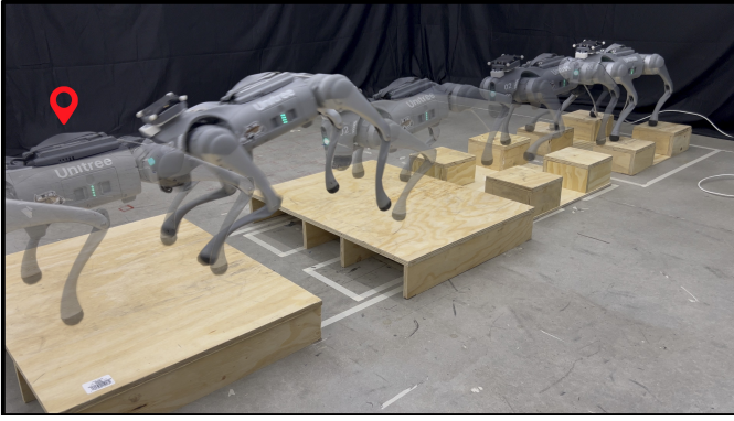
Fig. 12. Hardware experiment demonstration for the second unstructured terrain scenario with sparse stepping stones, flat, and gap terrains.
